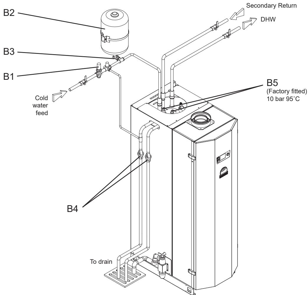
**6 Bar Unvented Kit c/w Through Flow Valve. Part No. 7726954
