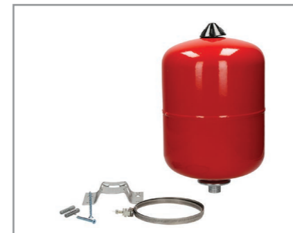
7210823 EXPANSION VESSEL 8L WITH BRACKET • Maximum working pressure of 10bar • 3/4" hydraulic connection • Air valve for re-charging
